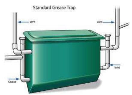
Please note: We've omitted the support stand, the steps and the work platform from the drawing for clarity. The design of the lid(s) for an above ground grease trap will vary between different manufactures.
